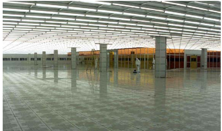
High Technology manufacturing areas mandate a clean room environment with low ambient noise.
