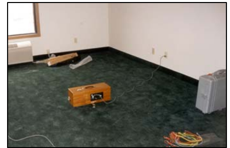
Impact Isolation Testing: Floor/Ceiling Construction New & Remediation
